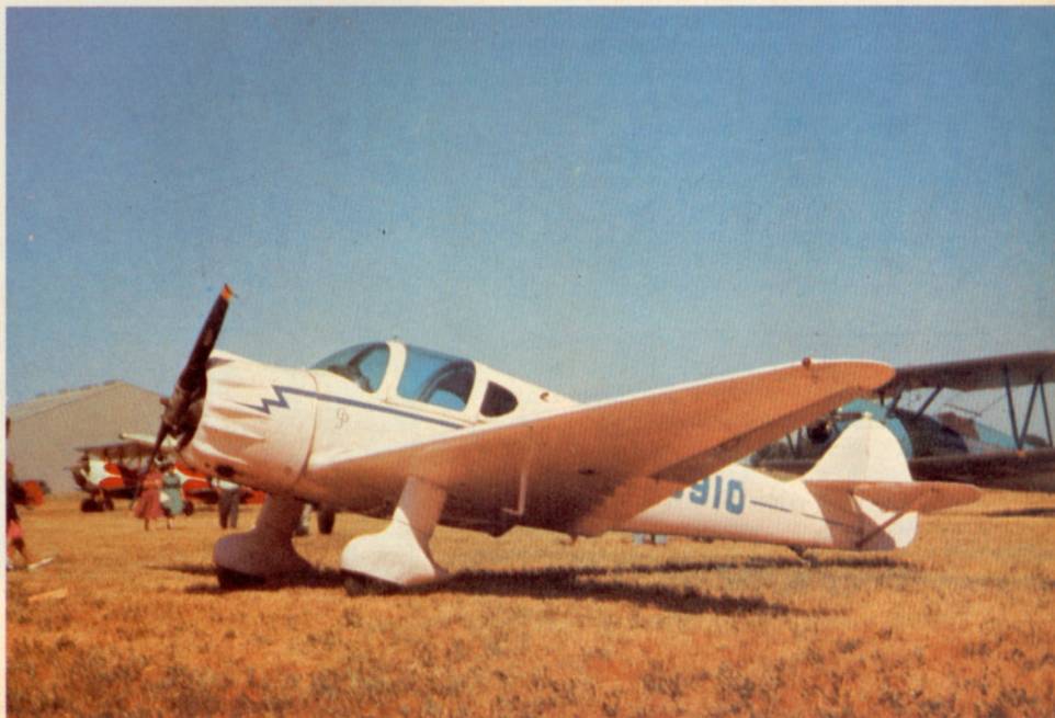
RYAN SCW 145 (1938), powered by Warner Super Scarab engine; top speed 152 m.p.h.; service ceiling 19,400 feet.
