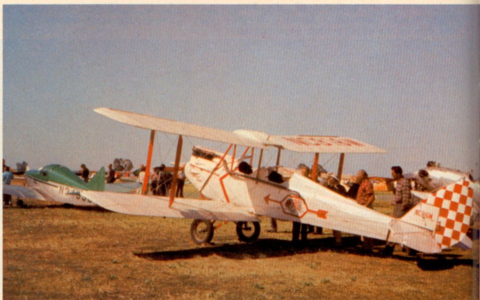
1929 deHavilland GYPSY MOTH, owned by Ed Clark, Jr., of Hawthorne, Calif., powered by a 100 h.p. D.H. Gypsy inline inverted engine.
