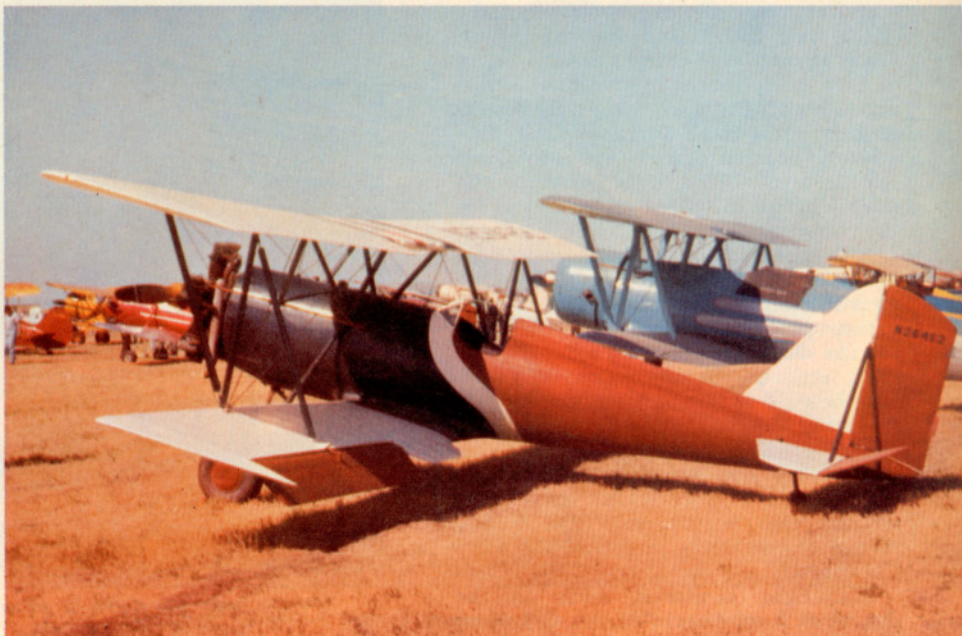
MEYERS OTW 160 (1942), powered by a 125 h.p. Warner engine; top speed rated at 120 m.p.h.; service ceiling 17,500 feet.
